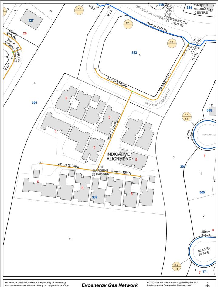
All network distribution data is the property of Evoenergy and no warranty as to the accuracy or completeness of the information is provided. No liability for any loss or damage arising from the use of this information will be accepted. Copyright © Evoenergy 2018.
